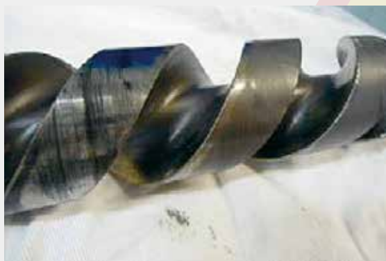
Example of trouble for 3 screw pump Damaged rotor
