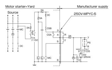
NOTE: Supply source to this system containing 30VA margin on the Tr.( Transformer )
