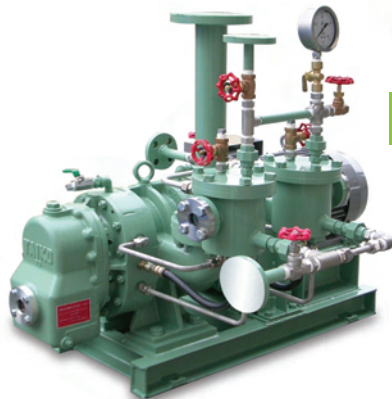
1 Stage Pressurized Gas Blower Sealing: 4-W mechanical seal Gas sector: Kanigen plating R-NZ Series (Direct drive motor)
